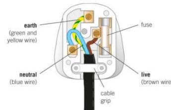
Figure 2 Inside a three-pin plug
