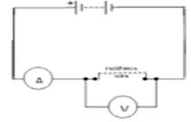
$$\text{resistance in } \Omega = \frac{\text{potential difference in V}}{\text{current in A}}$$
